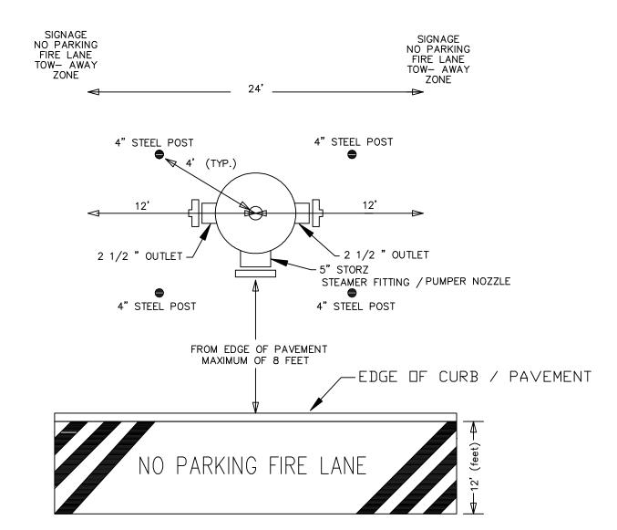
FIRE LANE TO BE 12 'IN DEPTH FROM EDGE OF PAVEMENT OR CURB. LETTERS TO BE 3' IN HEIGHT & MINIMUM OF 4" WIDE. STRIPPING TO BE MINIMUM OF 4" WIDE @ 45 DEGREE ANGLE & 5' ON CENTER. ALL MARKINGS TO BE TRAFFIC WHITE. SIGNAGE TO READ "NO PARKING FIRE LANE TOW AWAY ZONE. SIGNAGE TO MEET UNIFORM TRAFFIC CONTROL DEVICES MANUAL
